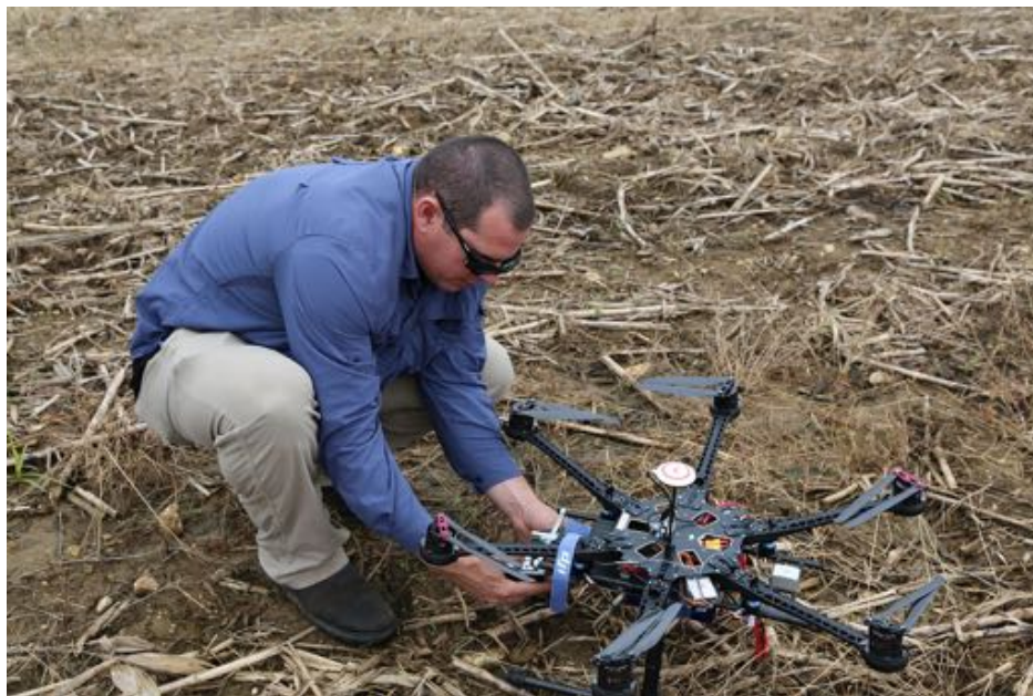
Figure 5.2 Prepping the S900 hexakopter for mapping (photo by M. Willis).
