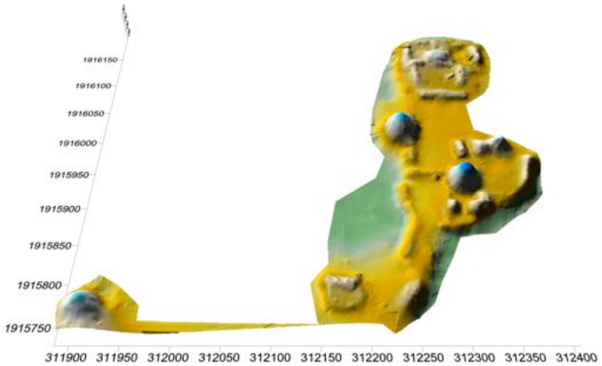
Figure 4.3 3D surface generated from the total station data using Surfer 12.
