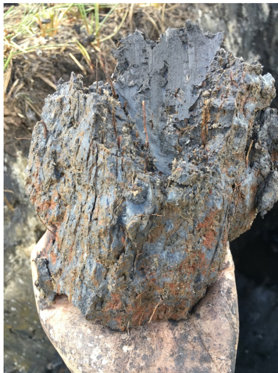
Figure 11.3 Example of redoxmorphic features along the ped faces and along root pathways within the upper vertic soil sequences (Photo by S. Krause).
