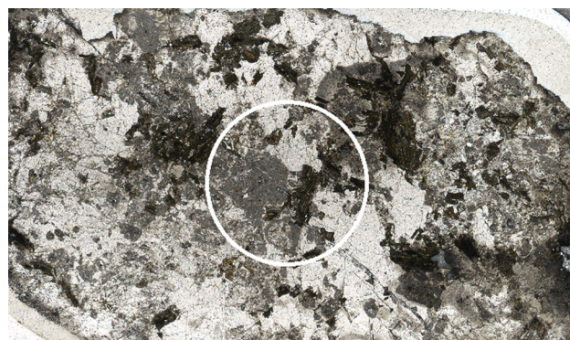
FIGURE 2 Scaled comparison of the 10 mm pXRF beam diameter compared to a 3.5 cm long petrographic thin section of CCB granite. CCB, Cockscomb Basin; pXRF, portable X-ray fluorescence.
