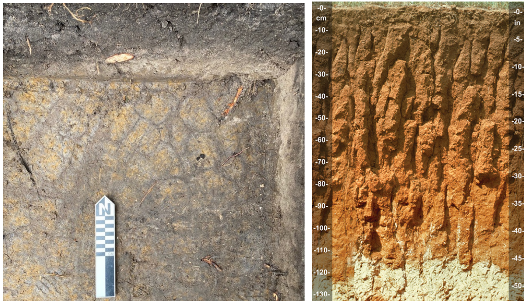
Figure 5.8 Prismatic soil structure seen (on the left) from above and (on the right) in cross-section (left photo by M. Brouwer Burg; right photo from Natural Resources Conservation Service [nrcs.usda.gov]).
